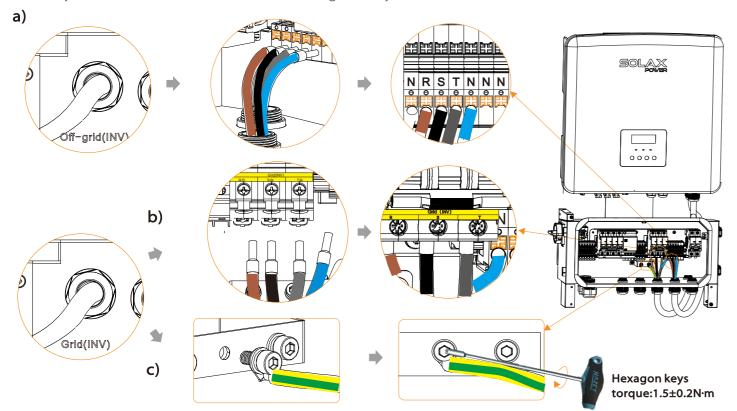
2) PV(PV1+/PV1-/PV2+/PV2-) /Gird(L1/L2/L3/N/PE) /Load(L1/L2/L3/N) side connection
