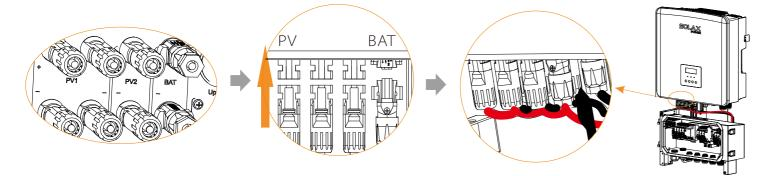
$\times$ Note: X3-Hybrid-5.0-M and X3-Hybrid-6.0-M inverters have only two MPPT and two PV strings, so when connecting, you need to unplug 1/2 of the PV in the X3-Matebox.
