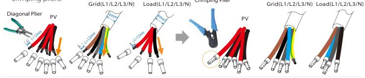
b) Gird(PE) strip the grounding cable insulation(lenhth"L), insert the stripped cable into the R type terminal, and then clamp it.
