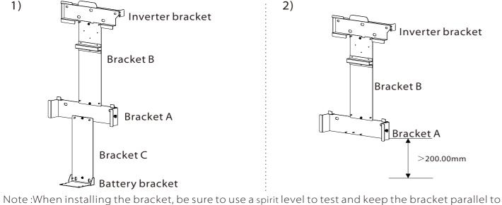
the horizontal plane. Bracket A should be installed at a distance of 200mm (at least) from the earth. Step 1: Splicing bracket
