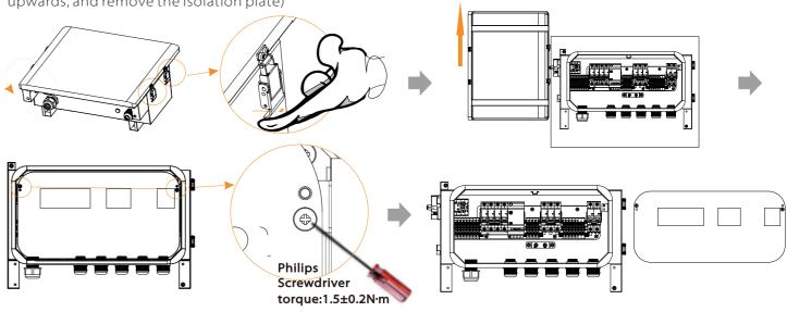
d) Mount X3-Matebox on bracket A and tighten the screws.
