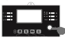
Step 4. Be sure to select battery type as "SOL" in LCD program 5.
