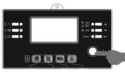
Step 4. Be sure to select battery type as "WEC" in LCD program 5.
