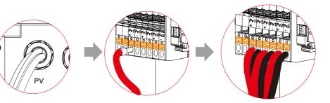
XNote: For X3-Hybrid-5.0-M and X3-Hybrid-6.0-M, there is only one PV1 line, and PV1+/PV1- corresponds to any pair of PV1+/PV1-ports on X3-Matebox.
