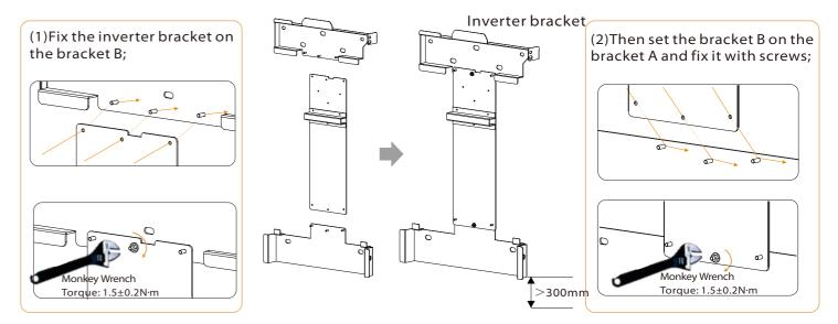
Note :When installing the bracket, be sure to use a spirit level to test and keep the bracket parallel to the horizontal plane.
