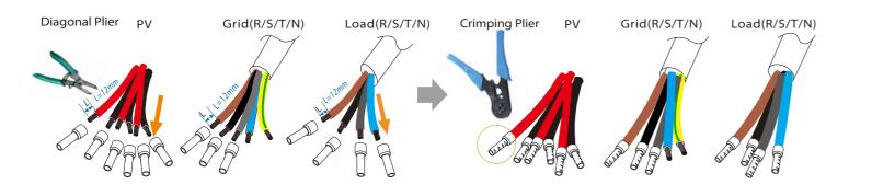
b) Grid(PE) strip the grounding cable insulation(length"L"), insert the stripped cable into the R type terminal, and then clamp it.
