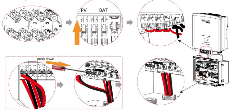
Note: X3-Hybrid-5.0-M and X3-Hybrid-6.0-M inverters have only two MPPT and two PV strings, so when connecting, you need to unplug (1/2) of the PV in the X3-Matebox. -Use a screwdriver to press down the yellow part while pulling the wire out of the port..
