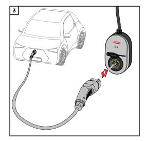
Connect a Type 2 to Type 2/Type 1 charging cable to the Wattpilot and the car.
