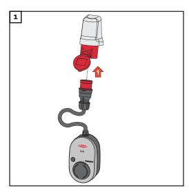
Connect the CEE plug to a suitable socket directly or with a suitable adapter.
