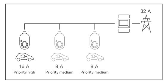
Distribution of the charging current with three Wattpilots with different priorities (one with high priority, two with medium priority).
