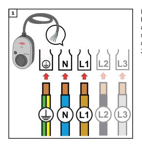
Have the 5-pin mains cable connected by an authorised electrician in accordance with national standards and safety rules. Depending on the available mains supply type, opt for a 1- or 3-phase connection.
