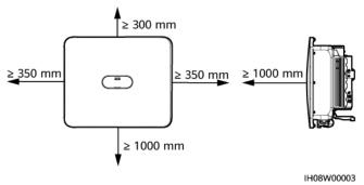
• When installing multiple inverters, install them in horizontal mode if sufficient space is available and install them in triangle mode if no sufficient space is available. Stacked installation is not recommended.
