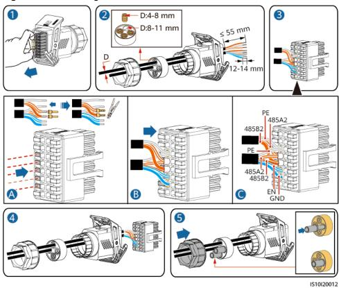
Figure 5-33 Installing cables
