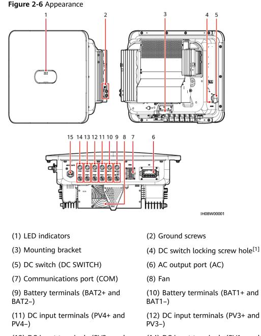
(13) DC input terminals (PV2+ and PV2-)
