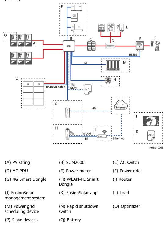
**Figure 2-2** Smart Dongle networking (the components in dashed boxes are optional)
