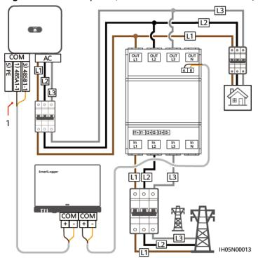
Figure 5-27 Three-phase, three-wire direct connection (SmartLogger networking)
