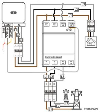
Figure 5-25 Three-phase, three-wire direct connection (Smart Dongle networking)
