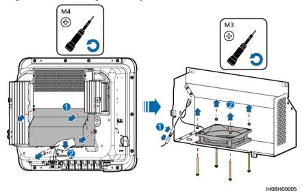
Step 2 Install a new fan, connect and bind the cables, and install the fan cover.
