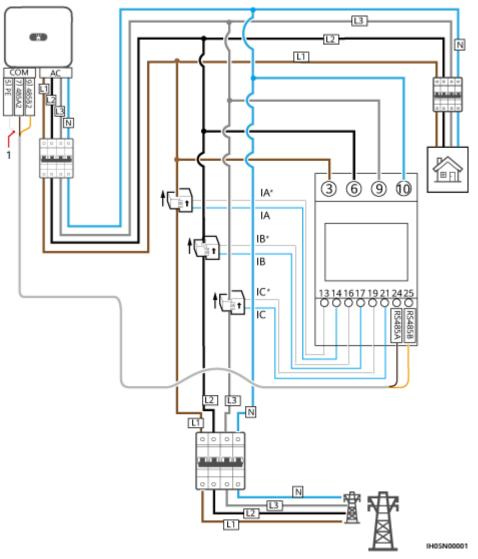
Figure 5-24 Three-phase, four-wire connection (Smart Dongle networking)
