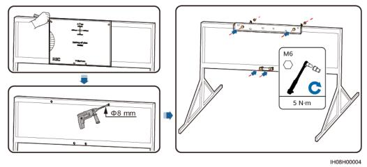
Step 4 (Optional) Install the DC switch locking screw.
