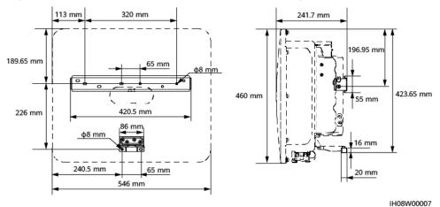
Figure 4-1 Dimensions of the inverter and mounting bracket
