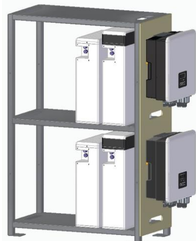
modul 1 x 46 kWh / 1 x 15 kW (46 kWh / 14 kW)
