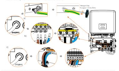
2) Grid (L1/L2/L3/N/PE) /Load (L1/L2/L3/N) side connection a) Prepare ordinary 6 mm $^2$  Grid (L1/L2/L3/N/PE) /6 mm $^2$  Load (L1/L2/L3/N) cable, remove 12 mm insulation layer from the end of the cable. And insert the European-style terminals respectively. The stripped terminals must be inserted into the European-style terminals and pressed down with the
