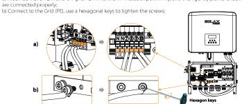
2) PV(PV1+/PV1-/PV2+/PV2-) /Gird(L/N/PE) /Load(L/N) side connection
