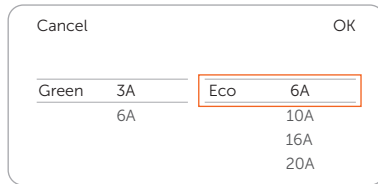
Figure 9-12 Charging current level for Eco mode
