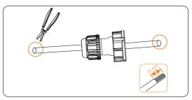
Figure 7-65 Stripping the communication cable for CT
