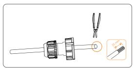
Figure 7-67 Stripping the communication cable for meter
