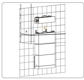
Figure 6-47 Placing the BMS
