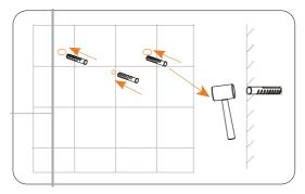
Figure 6-58 Knocking expansion tubes into the wall
