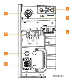
Figure 2-14 Ports of an inverter Table 2-8 Description of ports
