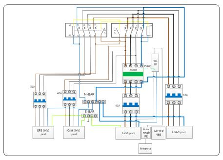
Figure 7-100 Matebox wiring diagram (with Wi-BR)
