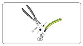
Figure 7-113 Stripping the PE cable
