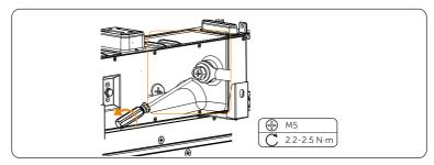
Figure 12-18 Disconnecting grounding cable
