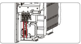
Figure 7-46 Well connected PV cables
