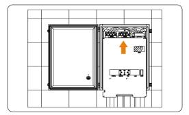
Figure 7-138 Reinstalling the plate
