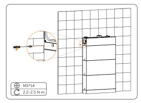
Figure 6-23 Tightening M5 screws
