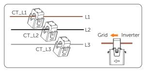
Figure 14-2 Clipping CTs to grid cables
