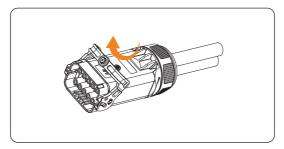
Figure 7-29 Pulling up the latch
