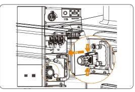
Figure 12-14 Disconnecting the communication connector
