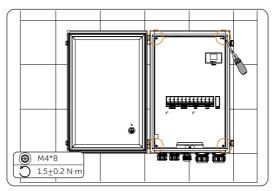
Figure 7-89 Loosening screws on the plate
