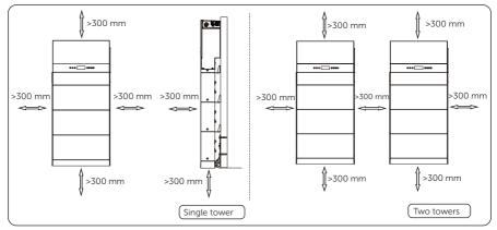
Figure 4-6 Clearance requirement
