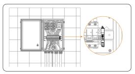
Figure 7-97 Installing the Wi-BR
