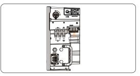
Figure 7-30 Removing the dustproof cover
