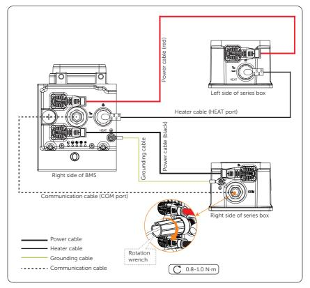
Figure 7-9 Connecting cables
