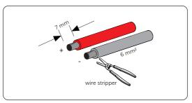
Figure 7-36 Stripping PV cables
