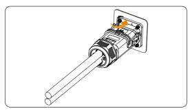
Figure 12-10 Loosening the AC connector
