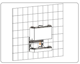
Figure 6-37 Placing battery module
