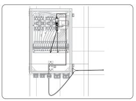
Figure 7-94 Connecting the Wi-BR and antenna
