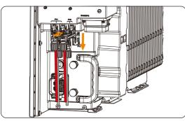
Figure 12-8 Pulling out PV dustproof buckles
