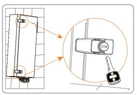
Figure 7-86 Unlocking the buckles
