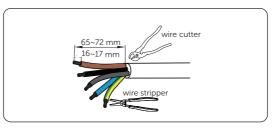
Figure 7-20 Striping the Grid and EPS cables
