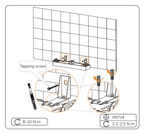
Figure 6-11 Securing the assembled bracket
