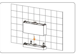
Figure 6-12 Placing the battery module
