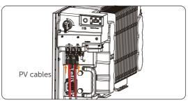
Figure 7-44 Connecting PV cables
