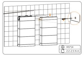
Figure 7-13 Tightening M5 screws
