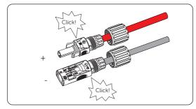
Figure 7-40 Securing PV cables
