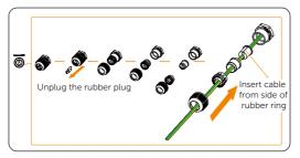
Figure 7-115 Threading the PE cable through Antenna&PE port
