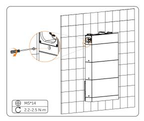
Figure 6-48 Tightening M5 screws
