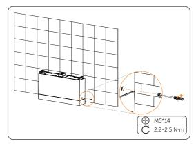
Step 10: Insert and tighten M5\*14 screws on both sides (torque: 2.2-2.5 N·m).
