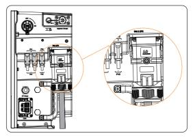
Figure 7-19 Well connected Grid & EPS cables
