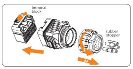
Figure 7-55 Disassembling the communication connector
