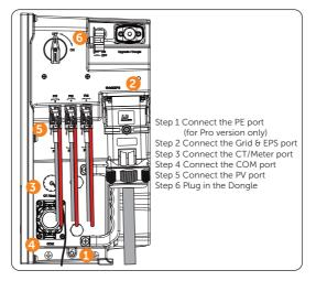
Figure 7-14 Wiring sequence of the inverter
