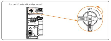
Figure 8-7 Turning off DC switch
