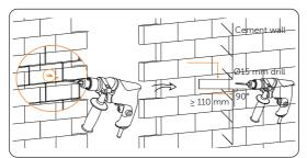
Figure 6-34 Drilling holes
