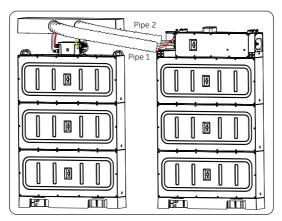
Figure 7-11 Inserting pipes into the cover
