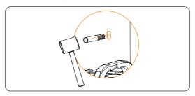
Figure 6-10 Inserting the expansion bolt
