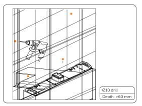
Figure 6-19 Drilling holes
