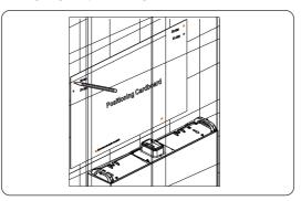
Figure 6-43 Marking the position of the brackets of the inverter
