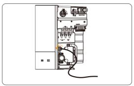
Figure 12-15 Disconnecting the CT/Meter cable
