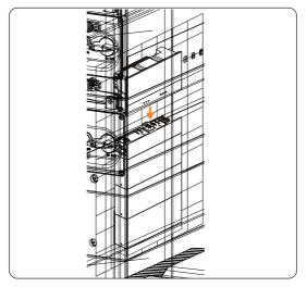
Figure 6-51 Installing the inverter
