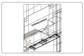
Figure 6-42 Aligning the positioning cardboard with the dots on the wall
