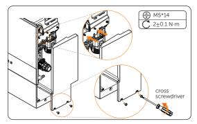
Figure 7-70 Locking the cable shielding board
