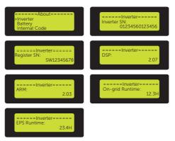
Figure 9-103 Displaying the inverter information
