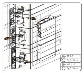
Figure 6-53 Locking the inverter brackets
