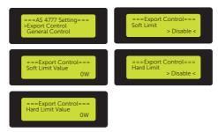
Figure 9-70 Setting export control in AS4777 setting interface
