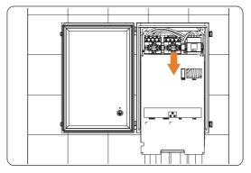
Figure 7-88 Removing the plate
