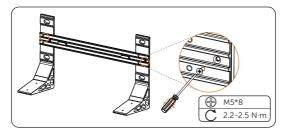
Figure 6-32 Attaching base support and transverse plate
