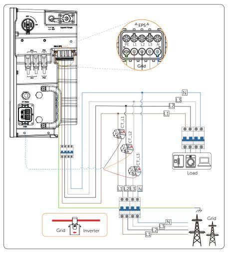
Figure 14-1 System wiring with CT
