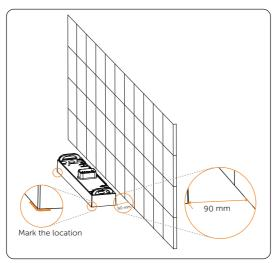
Figure 6-6 Placing the base
