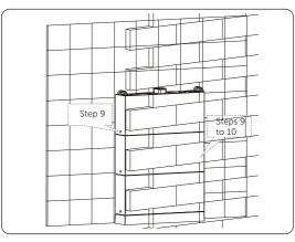
Figure 6-14 Placing battery modules
