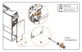
Figure 7-72 Locking the cable shielding board
