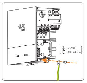
Figure 7-18 Securing the PE cable
