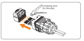
**Step 6:** Crimp ferrules and plug well crimped wires into the terminal block as needed.
