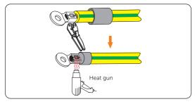
Figure 7-17 Crimping the cable
