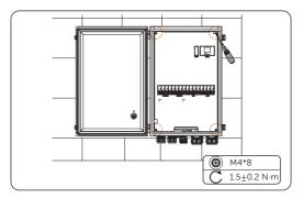
Figure 7-137 Securing the plate
