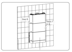
Figure 6-39 Placing battery modules
