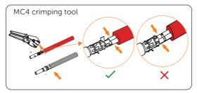
Figure 7-38 Crimping cables with PV pin contacts
