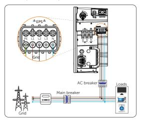
Figure 8-1 Turning on AC breaker
