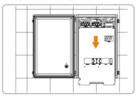
Figure 7-90 Removing the plate
