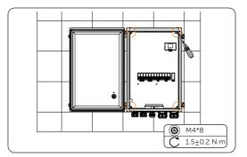
Figure 7-139 Securing the plate
