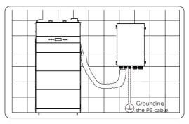
Figure 7-119 Connecting the PE cable to ground
