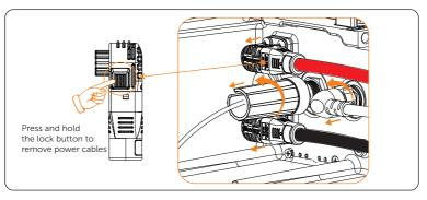
Figure 12-17 Disconnecting battery connectors
