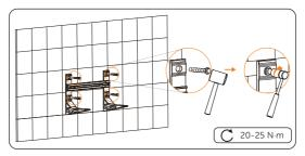
Figure 6-35 Tightening expansion screws
