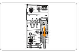
Figure 12-12 Unplugging the AC connector
