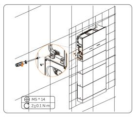
**Step 16:** Lock the screws on both sides of the inverter with the BMS.
