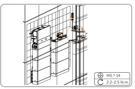
Figure 6-30 Placing the series box
