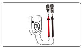
Figure 12-9 Measuring the voltage of PV connectors
