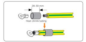
Figure 7-16 Inserting the stripped section into OT terminal
