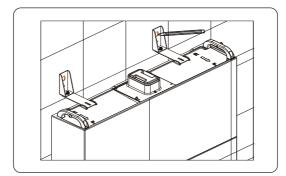
Figure 6-41 Marking the position of BMS
