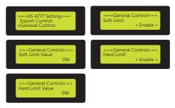
Figure 9-71 Setting general control in AS4777 setting interface
