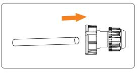
Figure 7-64 Threading the communication cable
