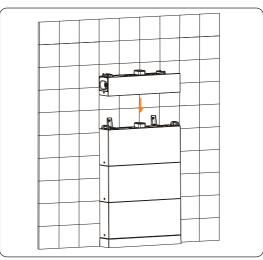
Figure 6-22 Placing the BMS
