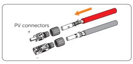
Figure 7-39 Threading PV cables with PV pin contacts connected
