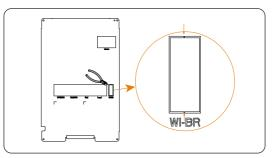
Figure 7-96 Cutting the baffle
