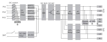
Figure 2-24 X3-IES-P system circuit diagram
