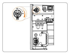
Figure 8-2 Turning on the DC switch
