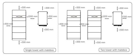
Figure 4-7 Clearance requirement with matebox
