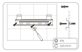
Figure 6-59 Securing the bracket
