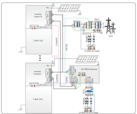
» Diagram 1: System diagram with SolaX X3-PBOX device
