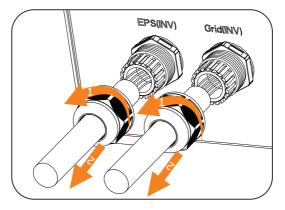
Figure 12-19 Disassembling EPS(INV) and Grid(INV) cables
