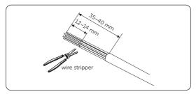
Figure 7-58 Stripping cables
