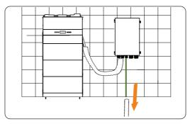
Figure 7-118 Inserting PE cable into the corrugated pipe
