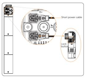
Figure 7-6 Removing short power cable
