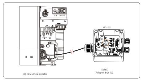
Figure 7-53 Inverter connected with a SolaX Adapter Box  $\mbox{G2}$
