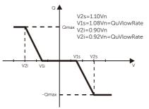
Figure 9-60 Curve Q=f(V)
