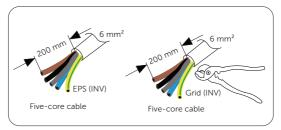
Figure 7-106 Stripping the EPS (INV) and Grid (INV) cable
