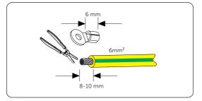
Figure 7-15 Striping the PE cable
