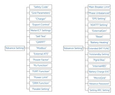
Figure 9-7 Advance setting diagram
