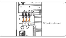
Figure 7-43 Removing the dustproof cover
