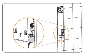
Figure 7-74 Installing the padlock
