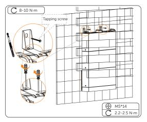
Figure 6-46 Securing the assembled bracket
