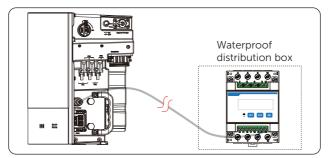
Figure 14-13 Connecting inverter to meter
