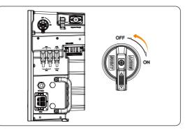
Figure 12-2 Turning off the DC switch
