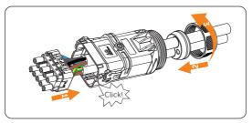
Figure 7-28 Wiring the AC connector
