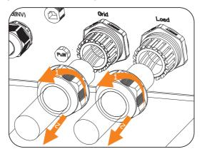
Figure 12-20 Disassembling Grid and Load cables
