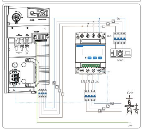
Figure 14-5 System wiring with direct-connected meter
