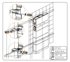
Figure 6-28 Locking the inverter brackets
