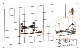
Figure 6-36 Securing the base
