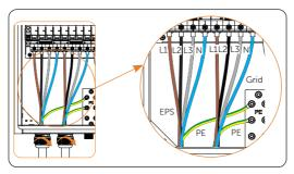
Figure 7-105 Connecting cables to the terminal block in the matebox
