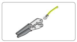
Figure 7-114 Crimping the PE cable
