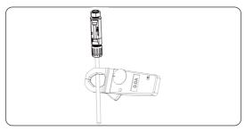
Figure 12-4 Detecting the current
