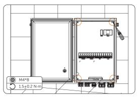
Figure 7-87 Loosening screws on the plate
