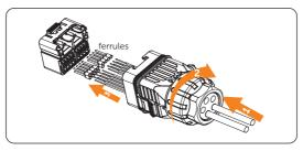
Figure 7-59 Inserting wires into ferrules
