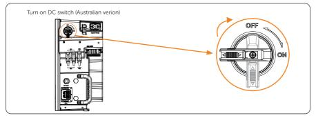
Figure 8-6 Turning on DC switch
