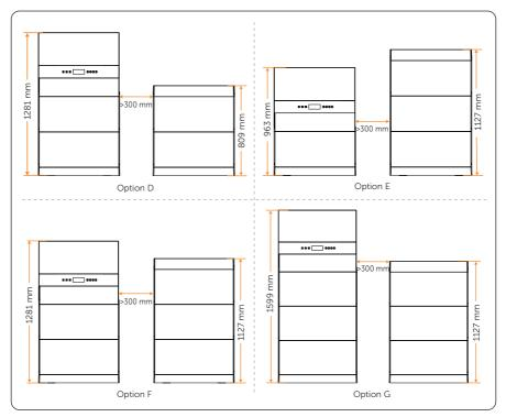
Figure 4-4 Installation options for two towers
