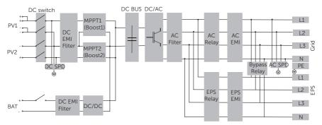
Figure 2-23 X3-IES system circuit diagram
