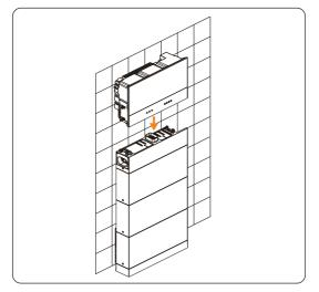
Figure 6-26 Installing the inverter
