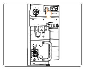
Figure 8-4 Pressing the inverter button
