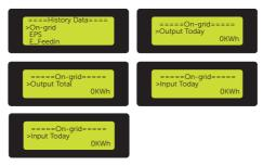
Figure 9-20 Displaying on-grid data
