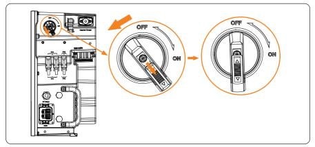
Figure 8-9 Unlocking DC switch
