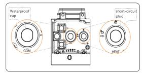
Figure 7-7 Removing waterproof cap
