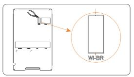
Figure 7-91 Cutting the baffle
