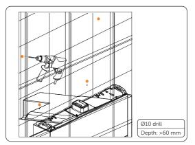
Figure 6-44 Drilling holes
