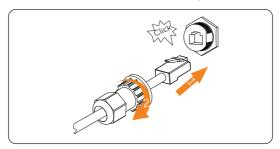
Figure 7-69 Connecting cable to the CT/Meter port
