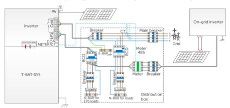
Figure 2-29 Micro grid system diagram
