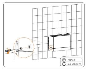
Figure 6-38 Tightening screws
