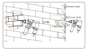
Figure 6-9 Drilling holes
