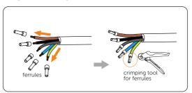
Figure 7-21 Crimping the Grid and EPS cables
