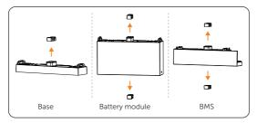
Figure 6-31 Removing dust covers
