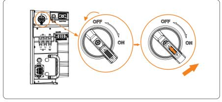
Figure 8-8 Locking DC switch
