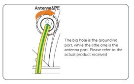
Figure 7-116 Tighting the waterproof connector
