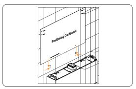
Figure 6-17 Aligning the positioning cardboard with the dots on the wall
