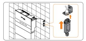
Figure 7-84 Plugging the dongle
