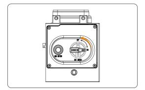
Figure 12-3 Turning off the BAT switch
