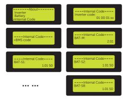
Figure 9-105 Displaying the internal code information
