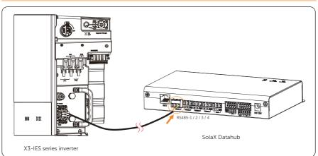
Figure 7-51 Inverter connected with a SolaX datahub
