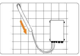
Figure 7-111 Inserting EPS and Grid cables into the corrugated pipe
