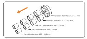
Figure 7-24 Taking out sealing plug
