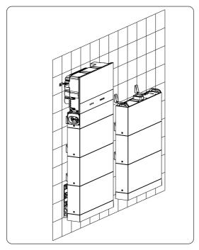
Figure 6-54 Installing two towers
