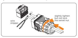
Figure 7-56 Stripping cables
