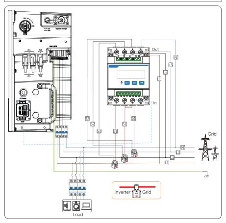
Figure 14-10 System wiring with CT-connected meter
