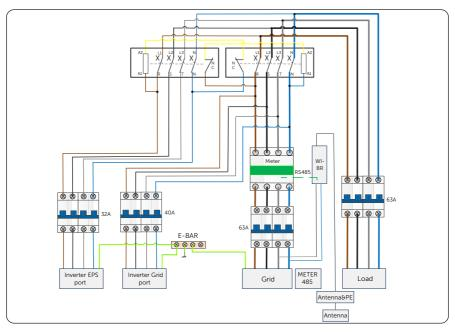
Figure 7-95 Matebox wiring diagram (with Wi-BR)
