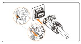
Figure 7-31 Plugging the AC connector into the port on the inverter
