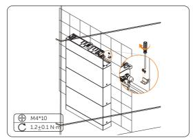
Figure 6-49 Install the anti-tamper bracket
