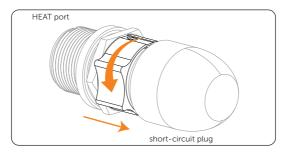
Figure 7-8 Closing short-circuit plug
