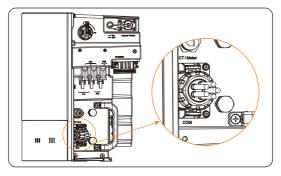
Figure 7-54 Well connected COM port
