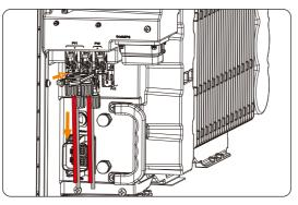
Figure 12-7 Pulling out PV connectors
