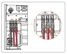
Figure 7-35 Well connected PV cables
