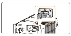
Figure 7-82 Installing the WiFi connecting cable
