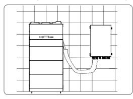
Figure 7-112 Well connected EPS and Grid cable
