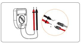
Figure 7-42 Measuring the voltage of PV connectors
